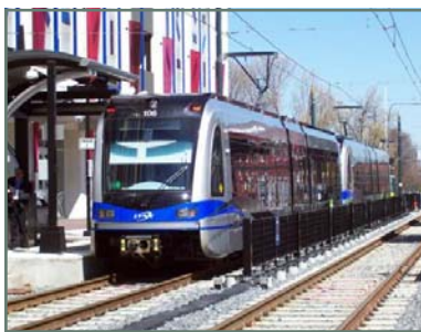
Light Rail, Charlotte, NC: includes light-weight passenger rail cars traveling singly or in short two-car trains on a fixed right-of-way, usually not separated from on-street traffic for much of the way.
