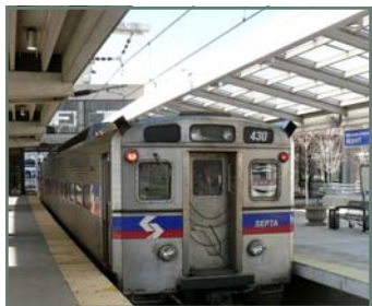
Heavy Rail, Philadelphia, PA: includes metros, subways, and rapid rail systems; usually with multiple-car trains on fixed, exclusive rights-of-way.
